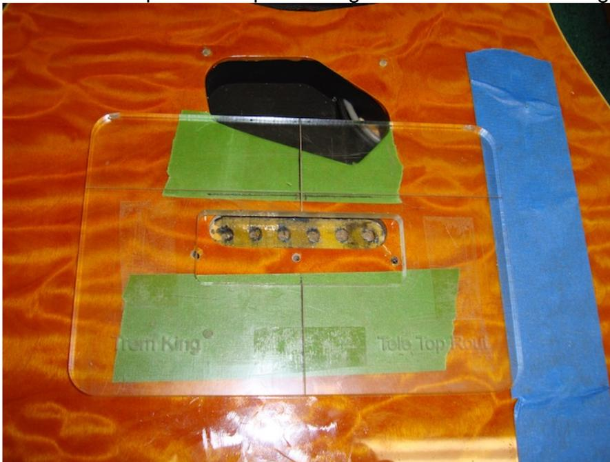
4. **Cut Top Rout.** Use plunge router with bit # 45491,  $\frac{3}{4}$ " bit to start the rout.
